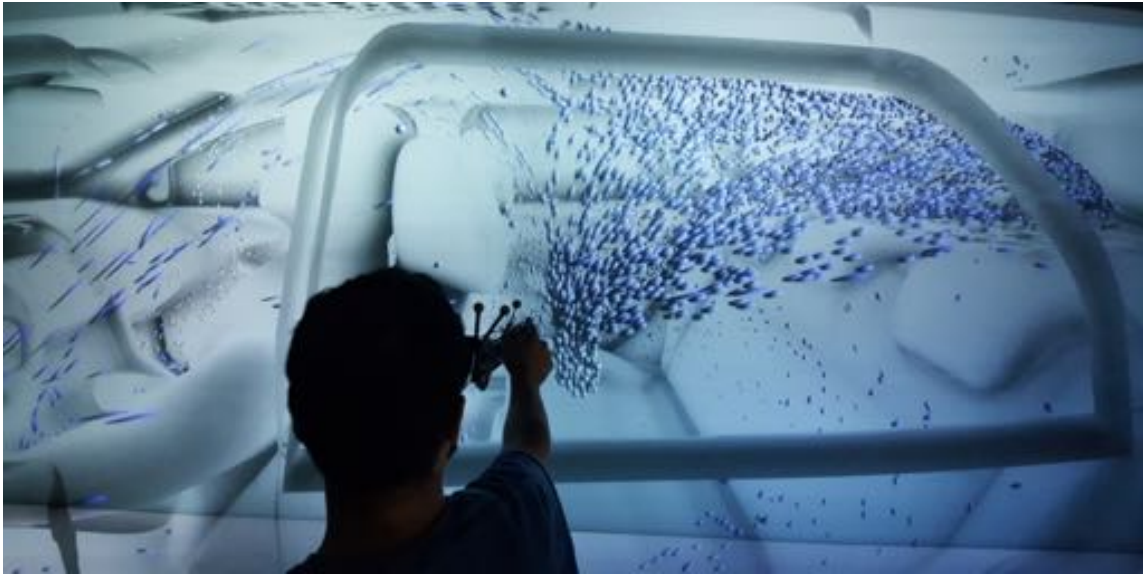
Figure 21.7: Inside the same vehicle as Figure 21.6, a user interactively explores the airflow inside an electric vehicle cabin, by directly seeding particles into the flow. Using this VR system, engineers were able to identify flow characteristics they had not discovered using desktop visualization tools.
